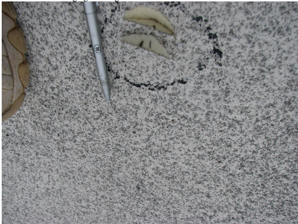
Photo 2 Slit samples can show the severity of damage from hail impact. The crack in this sample is less than 1/4 inch indicating light damage
